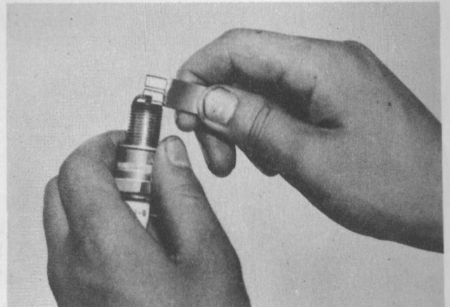
Fig. 6-92 Adjusting Gap W0544
