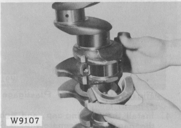
Fig. 2-60 Installing Plastigage
