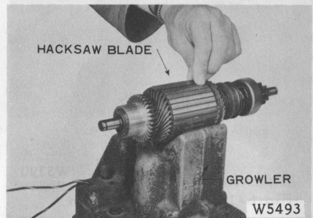
Fig.6-14 Armature Core Test
