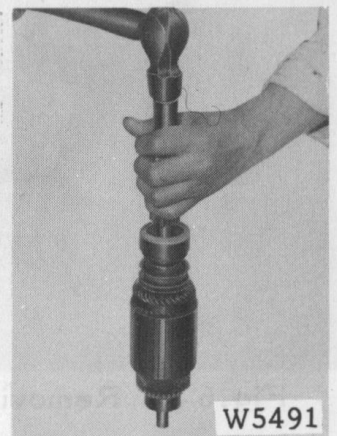
Fig.6-12 Starter Clutch Removal
