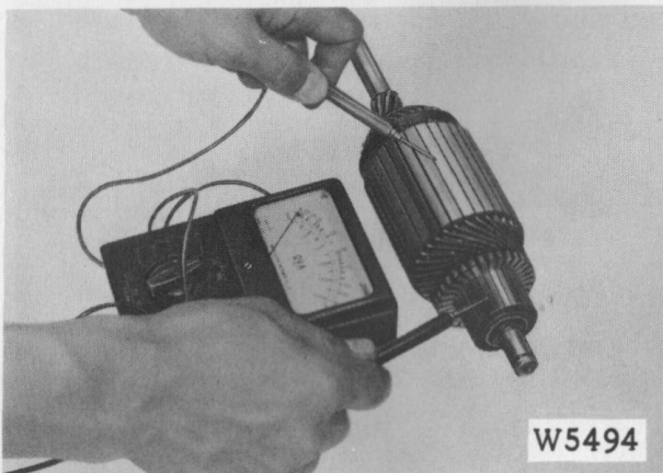
Fig. 6-15 Commutator Short Test
